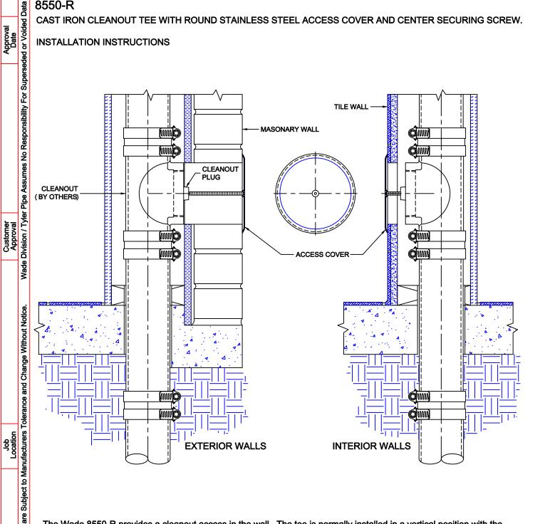
The Wade 8550-R provides a cleanout access in the wall. The tee is normally installed in a vertical position with the cleanout facing the wall. The wall access cover is used to cover the cleanout plug. The round access cover is mounted on the surface of the finished wall and is secured by the screw to a tapping which is provided in the cleanout plug. A 3-1/2" long 1/4-20NC screw is provided - screw may require field cutting to exact length as application demands.
