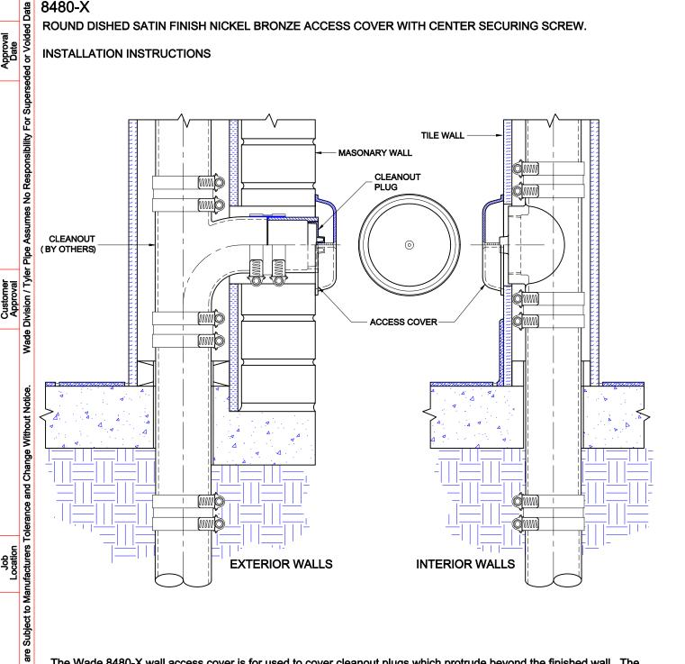
The Wade 8480-X wall access cover is for used to cover cleanout plugs which protrude beyond the finished wall. The round access cover is mounted on the surface of the finished wall and is secured by the screw to a tapping which must be provided in the cleanout plug. A 3-1/2" long 1/4-20NC screw is provided - screw may require field cutting to exact length as application demands.
