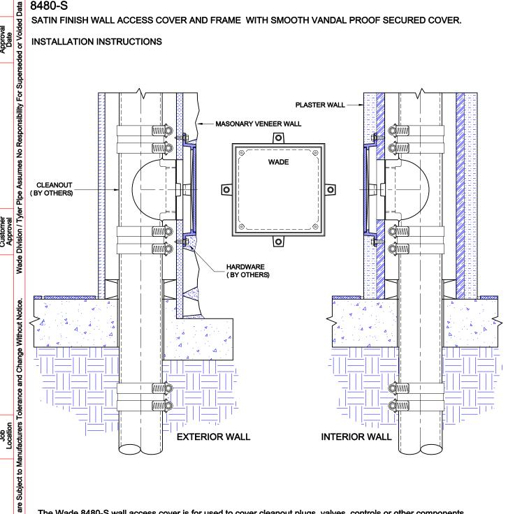
The Wade 8480-S wall access cover is for used to cover cleanout plugs, valves, controls or other components concealed in walls. The square design lines up with adjacent wall and floor tiles. The mounting lugs provide an easy means of securing the frame to the wall construction.
