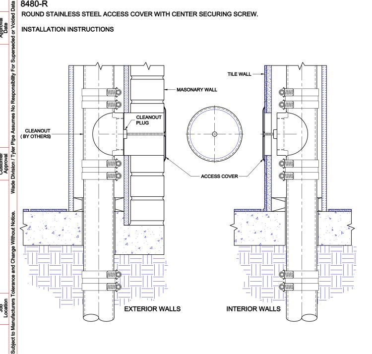
The Wade 8480-C wall access cover is for used to cover cleanout plugs concealed in walls. The round access cover is mounted on the surface of the finished wall and is secured by the screw to a tapping which must be provided in the cleanout plug. A 3-1/2" long 1/4-20NC screw is provided - screw may require field cutting to exact length as application demands.
