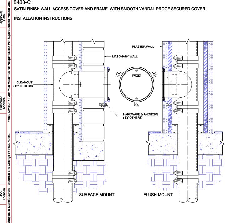
The Wade 8480-C wall access cover is for used to cover cleanout plugs, valves, controls or other components concealed in walls. The round design eliminates te necessity of lining up with adjacent floors, wallts, etc. The mounting lugs provide an easy means of securing the frame to the wall construction.
