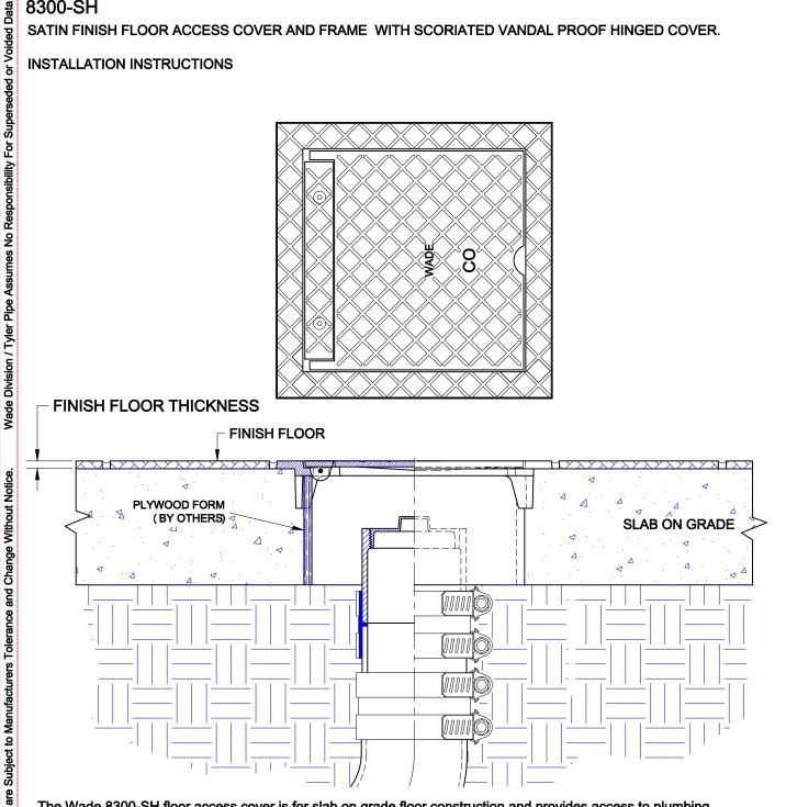
The Wade 8300-SH floor access cover is for slab on grade floor construction and provides access to plumbing cleanouts or other components. The drain piping is first run to an elevation below the expected finish floor level. The cleanout or other component is terminated below the finish floor level. The contractor provides a plywood form to house the cleanout and the 8300-SH access cover/frame provides the floor level access.
