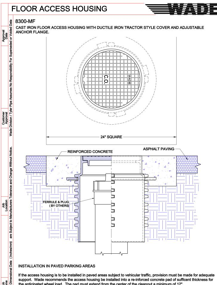
support. Wade recommends the access housing be installed into a re-inforced concrete pad of sufficent thickness for the anticipated wheel load. The pad must extend from the center of the cleanout a minimum of 12".
