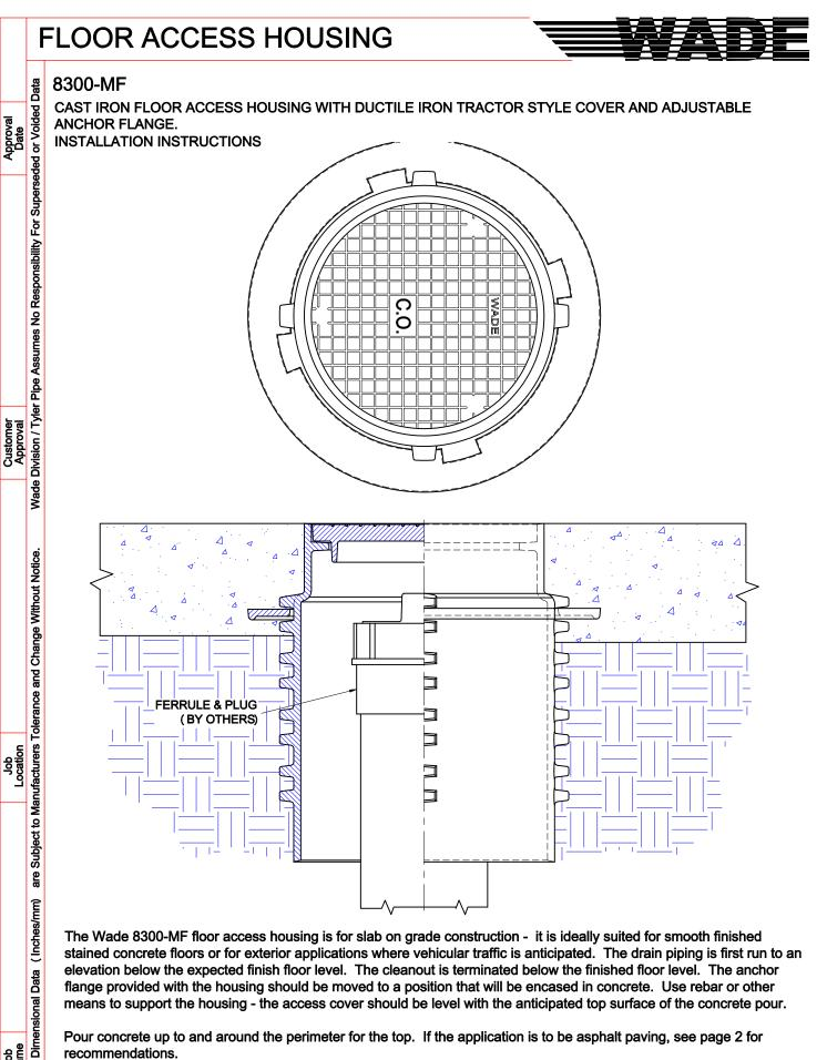
Pour concrete up to and around the perimeter for the top. If the application is to be asphalt paving, see page 2 for recommendations.
