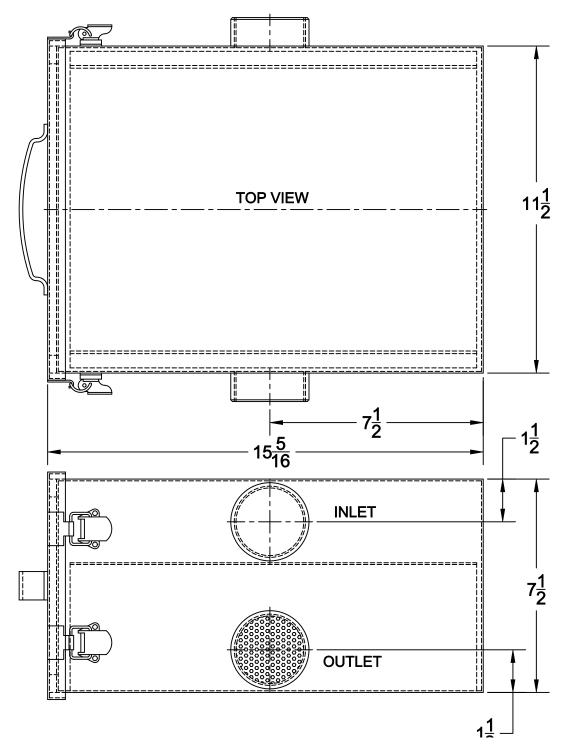
UNIT HAS INLETS/OUTLETS ON EACH SIDE FOR RIGHT OR LEFT HAND MOUNTING.
