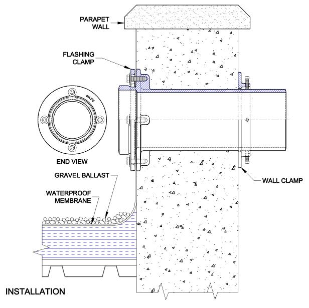
The Wade 3940-D parapet wall scupper sleeve serves as an emergency over flow scupper drain. Cut-off grooves in the sleeve body allow for field cut lengths to accommodate various wall thicknesses.
