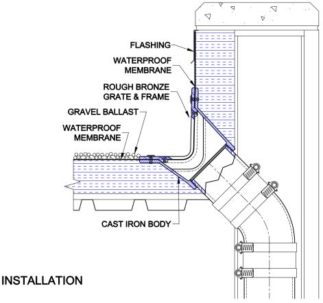
The Wade 3290-A is used at the junction of the roof and parapet. The side outlet (45°) allows the connected piping to be easily routed beside the wall. Tyler No-Hub pipe and fittings may be utilized.
