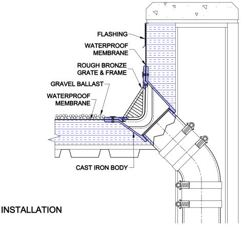
The Wade 3270-A is used at the junction of the roof and parapet. The side outlet (45°) allows the connected piping to be easily routed beside the wall. Tyler No-Hub pipe and fittings may be utilized. The oblique grate prevents debris from blocking drainage.
