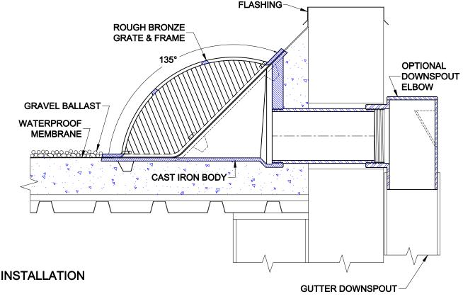
The Wade 3230-N is used at the junction of the roof and parapet. The side outlet (90°) may be connected to outside downspout by using a Wade 3940-DE downspout adaptor or if the piping is inside, Tyler No-Hub pipe and fittings may be utilized. The oblique grate prevents debris from blocking drainage.
