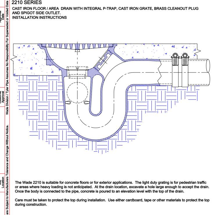
The Wade 2210 is suitable for concrete floors or for exterior applications. The light duty grating is for pedestrian traffic or areas where heavy loading is not anticipated. At the drain location, excavate a hole large enough to accept the drain. Once the body is connected to the pipe, concrete is poured to an elevation level with the top of the drain.
