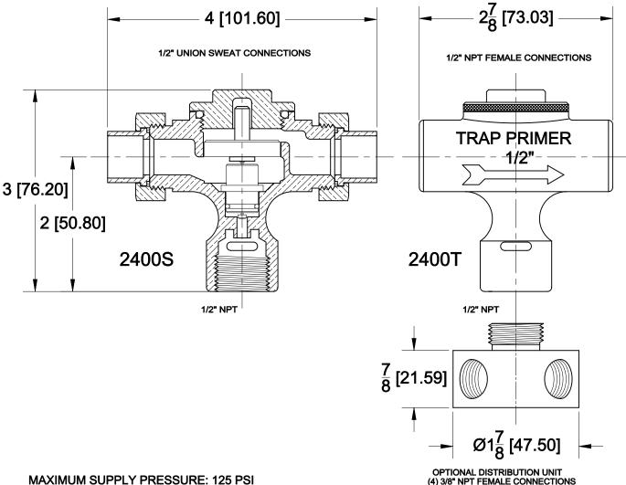
MAXIMUM SUPPLY PRESSURE: 125 PSI MINIMUM SUPPLY PRESSURE MUST EXCEED 25 PSI
