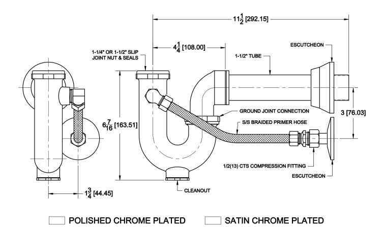
FUNCTION: The water saver trap primer utilizes the temporary "head" of water in the p-trap which occurs during use of lavatories, sinks and drinking fountains to overflow through the primer tube connection and thus gravity flow through piping under the floor to a floor drain trap primer connection, maintaining the trap seal.
